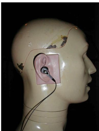
Figure 3. Placement of stereo inner-phones for  $H(EC_{SIP})$  measurements.
