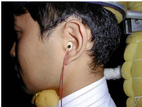
Figure 6. Placement of the ear-microphones for HRTF measurement.
