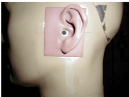
Figure 2. Placement of microphones for  $HRTF(EEC)$  measurements.
