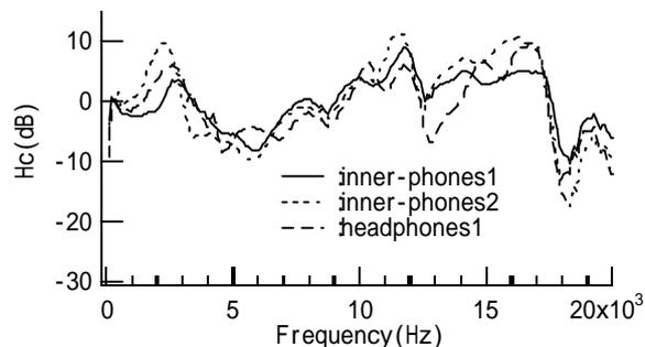
Figure 5. Examples of the obtained  $H_c$  of various kinds of inner-phones.
